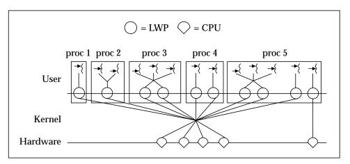
*Figure 3* Multithread Architecture Examples
